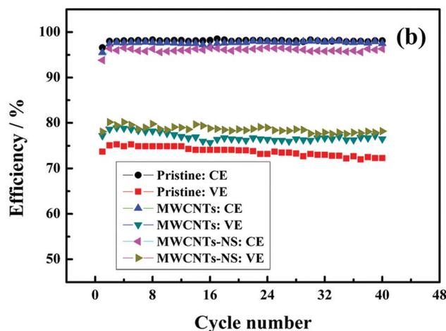
Fig. 7 The discharge capacity (a) and efficiency (b) of the cells using different MWCNTs samples as a function of cycle number at the current density of 50 mA cm<sup>-2</sup>.
