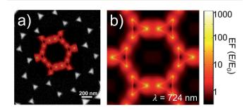
Fig. 4 (a) SEM image of sample S1-nOx and (b), and as inset in (a), simulated map of the local-field enhancement calculated at the indicated wavelength (corresponding to the maximum of the simulated absorbance spectrum).
