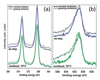
Fig. 6 Ag 3d spectra (a) and O 1s spectra (b) of silver films, both asdeposited and intentionally oxidized at 70 °C, 30 min in air.
