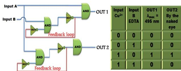
Fig. 9 Truth table and sequential logic circuits displaying memory units with two inputs (input A (Cu<sup>2+</sup>) and input B (EDTA)) and two outputs in the presence of chemical inputs.
