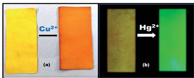
Fig. 11 (a) Naked eye detection on a piece of paper soaked with **FDNS**: from left to right **FDNS** (blank); **FDNS** +  $\text{Cu}^{2+}$  (b) the variation of the color of **FDNS** coated on filter paper before (left) and after treatment with  $\text{Hg}^{2+}$  (right) under UV excitation light.
