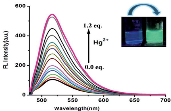
Fig. 5 Fluorescence spectral titrations of FDNS (10  $\mu\text{M}$ ) in aqueous : MeOH (8 : 2 v/v) HEPES buffer (1 mM, pH 7.4) on the incremental addition of  $\text{Hg}(\text{NO}_3)_2$  (1.2 equiv.)  $\lambda_{\text{ex}} = 465 \text{ nm}$ . Inset: the colour change of FDNS solution in the presence of  $\text{Hg}^{2+}$  ions under UV light.
