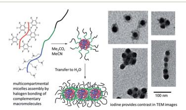
**Fig. 16** Micelles formed *via* halogen bonding between triblock copolymer and halogenbond donor polymer. Adapted from DOI: 10.1039/c7fd00111h with permission from The Royal Society of Chemistry.
