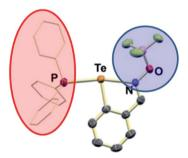
Fig. 13 N-Te···P chalcogen bond. Strong chalcogen bonding capability of Te is activated by coordination of N-oxide, and further enhanced by Lewis acid coordination of the BF $_3$  group to the oxygen (blue circle). Phosphine (PPh $_3$ , red ellipse) serves as the (Lewis basic) chalcogen bond acceptor. Adapted from DOI: 10.1039/c7fd00075h with permission from The Royal Society of Chemistry.
