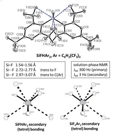
Fig. 11 Crystal structure of SiFHAr<sub>2</sub>,  $Ar = C_6H_2(CF_3)_3$  (top), with secondary (tetrel) bonding shown as dashed bonds. Primary bonding (solid lines) and secondary bonding (dashed lines) at Si in SiFHAr<sub>2</sub> and SiF<sub>2</sub>Ar<sub>2</sub> (bottom). Secondary (tetrel) Si···F bonds are longer than primary (covalent) Si–F bonds. Secondary bonds *trans* to F are shorter than those *trans* to C. Adapted from ref. 57 with permission from Elsevier.
