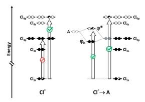
Fig. 6  $Cl_{1s}$  to  $Cl_{3p}$  transition, which can be probed by XAS, arises only if  $Cl_{3p}$  to  $I_2(\sigma^*)$  charge-transfer is present (A represents a halogen-bond acceptor, here  $I_2$ ). The intensity of the transition is proportional to the  $Cl_{3p}$  character in the  $\psi^*$  orbital. Reproduced from DOI: 10.1039/c7fd0076f with permission from The Royal Society of Chemistry.
