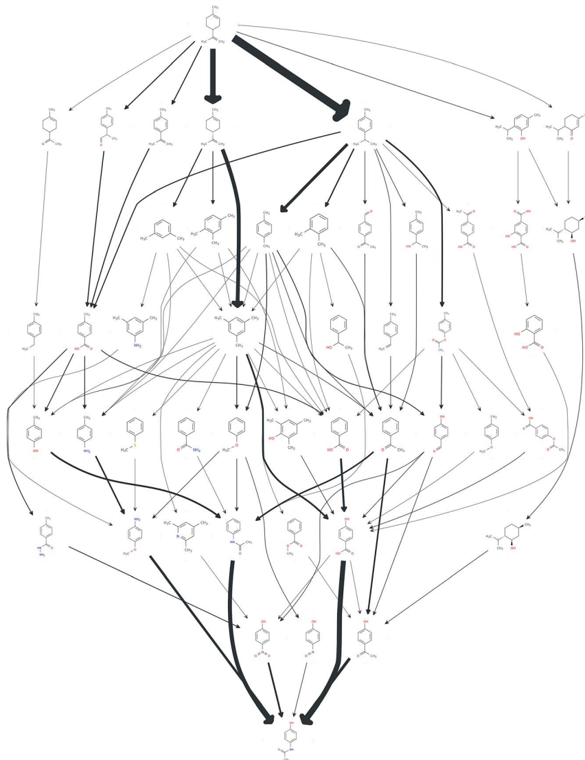
Fig. 1 A network of possible synthetic routes from limonene to paracetamol. The thickness of an edge corresponds to the number of times a route has been reported. The plot is for illustrative purposes and the nodes are positioned by an automated graph algorithm, thus their relative positioning does not necessarily contain any chemical insights.
