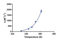
Fig. 5 Dependence of kinetic association constants on temperature. The data points were fitted to the Arrhenius equation.
