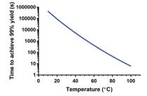
Fig. 6 Prediction of time needed to achieve 99% yield for  $[^{177}Lu]Lu$ -DOTA-TATE in a setup with optimal heat and mass transfer. The graph was calculated using the Arrhenius parameters obtained in this study.
