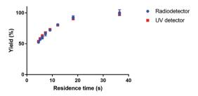
Fig. 3 Comparison of measured reaction yield of [ $^{177}$ Lu]Lu-DOTA-TATE for UV and radio-detection. The reaction was done in a 100  $\mu$ m channel at 80 °C.
