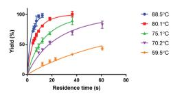
Fig. 4 Dependence of formation of Lu-DOTA-TATE on temperature. All reactions were done in a 100  $\mu m$  channel. The data points for each temperature were fitted to an equation representing second order kinetics.
