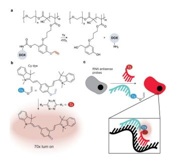
Fig. 56 (a) PEG polymer conjugated to a doxorubicin pro-drug through a self-immolative, which is eliminated upon reaction with tetrazine liberating the bioactive drug. (b) NIR-emitting vinyl ether cyanine dye activated by tetrazine reaction. (c) A fluorogenic NIR RNA-templated tetrazine uncaging probe could be used for cell imaging of mRNA
