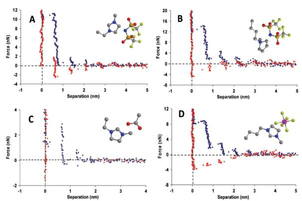
Fig. 3 Force-distance profile for a  $Si_3N_4$  AFM tip approaching (blue) and retracting from (red) a mica surface in (A)  $[C_2mim^+][NTf_2^-]$ , (B)  $[C_4mpyrr^+][NTf_2^-]$ , (C)  $[C_2mim^+][NTf_2^-]$ , and (D)  $[C_4mim^+][PF_6^-]$ . Reproduced from ref. 24 with permission from the PCCP Owner Societies.
