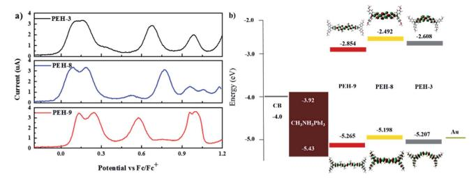
Fig. 3 (a) Differential pulse voltammetry (DPV) of the three compounds with 0.1 M tetrabutylammonium hexafluorophosphate in  $CH_2Cl_2$  at a scan speed of 50 mV s<sup>-1</sup>, potentials vs. Fc/Fc<sup>+</sup>; (b) energy level diagram of each component in a hybrid solar cell calculated based on DPV measurements with isodensity surface plots of PEH-3, PEH-8 and PEH-9 as calculated by time dependent-density functional theory (TD-DFT) using the B3LYP functional/6-31G\* basis set.
