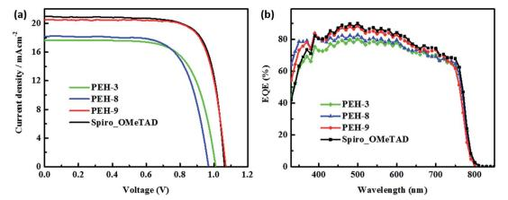
Fig. 5 (a) Current (J) –voltage (V) curves of the solar cells with PEH-3, PEH-8, PEH-9 and Spiro-OMeTAD control recorded from forward bias (FB) to short circuit conditions (SC) under AM 1.5 conditions (100 mW cm<sup>-2</sup>). (b) Incident photon-to-electron conversion efficiency (IPCE) as a function of wavelength for the PSCs in (a).
