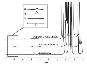
Fig. 2 <sup>1</sup>H NMR spectra of purified POEGMA-b-PVBA-GEN overlaid with POEGMA-b-PVBA and POEGMA
