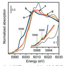
Fig. 9 Normalized XANES spectra of the 1.0-Cr/DHS sample after treatment under different propane dehydrogenation reaction conditions: a) only  $C_3H_8$  (green curve), b)  $C_3H_8 + CO_2$  (blue curve), c)  $C_3H_8 + O_2$  (red curve) and d)  $C_3H_8 + CO_2 + O_2$  (orange curve). The spectrum of Cr<sub>2</sub>O<sub>3</sub> is shown as a reference for comparison (grey curve)
