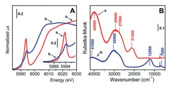
Fig. 4 Normalized XANES (A) and DR UV-Vis (B) spectra of the 0.5-Cr/ DHS catalyst in the dehydr/ox (curves a, red) and dehydr/red (curves b, blue) states. The insert in panel A shows an enlargement of the preedge region. In panel B, the sharp component labelled with an asterisk is due to the  $2v_{OH}$  vibration of silanols at the support surface.
