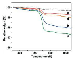
Fig. 7 Thermogravimetric analysis of the amount of coke formed on the 2.0-Cr/DHS catalyst after 400 min of ODH of propane reaction (T = 873 K,  $w = 200 \text{ h}^{-1}$ ) under different conditions: a)  $C_3H_8: N_2 = 15:85$ (green); b)  $C_3H_8:CO_2:N_2=15:30:55$  (blue); c)  $C_3H_8:O_2:N_2=15:3:$ 82 (red); d)  $C_3H_8: CO_2: O_2: N_2 = 15:30:3:52$  (orange).
