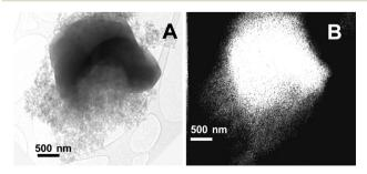
Fig. 3 TEM/EDS data obtained for the 2.0-Cr/DHS sample, representative of all catalysts: the image (A) and the corresponding EDS map of the Cr location (B) of an aggregate of the ordered and disordered porous phases. The difference in the brightness in the maps is mainly due to the difference in thickness of the analysed regions.
