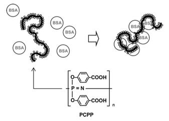
Fig. 21 A schematic representation of PCPP, a polyphosphazene-based polyacid, and the proposed conjugation with BSA (bovine serum albumin). Reprinted from A. K. Andrianov et al., Biomacromolecules, 2005, 6, 1375. Copyright 2005 American Chemical Society. 42
