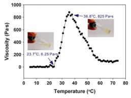
**Fig. 24** Temperature-dependent sol-gel transition and viscosity change of a suitably functionalised poly(organo)phosphazene. Adapted with permission from Y.-M. Kim *et al.*, *ACS Nano*, 2012, **6**, 5757. Copyright 2015 American Chemical Society. <sup>46</sup>
