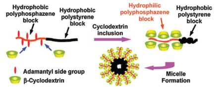
Fig. 15 In situ formation of amphiphilic polystyrene–polyphosphazene diblock copolymers via host–guest inclusion complexes with β-cyclodextrin can be used to prepare supramolecular aggregates. Reprinted with permission from S. Y. Cho and H. R. Allcock, Macromolecules, 2009, 42, 4484. Copyright 2009, American Chemical Society.<sup>34</sup>
