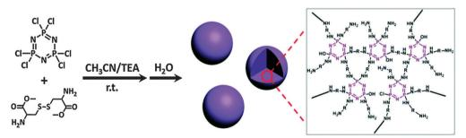
Fig. 19 An example of a precipitation condensation reaction to give cyclomatrix polyphosphazenes using [PNCl<sub>2</sub>]<sub>3</sub> as a building block. Adapted from Z. Huang et al., Chem. Commun., 2015, 51, 8373 with permission from The Royal Society of Chemistry.<sup>39</sup>
