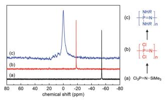
Fig. 4 Sample <sup>31</sup>P{<sup>1</sup>H} NMR spectra of the monomer trichlorophosphoranimine Cl<sub>3</sub>PNSiMe<sub>3</sub> (a), polydichlorophosphazene [NPCl<sub>2</sub>]<sub>n</sub> (b) and a macrosubstituted poly(organo)phosphazene [NP(NHR)<sub>2</sub>]<sub>n</sub> (c) demonstrating the simple tracking of the reaction progression. Adapted from H. Henke et al., J. Polym. Sci., Part A: Polym. Chem., 2013, 51, 4467. Copyright 2013 Wiley Periodicals, Inc. 12
