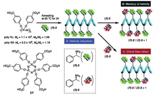
Fig. 17 Dynamic helicity of poly[di(4-carboxyphenoxy)phosphazene] and its application as a chirality filter. Note: the polymer referred to as Poly1L here is essentially PCPP, a well-known polyphosphazene investigated for use in medical applications. Reprinted with permission from K. Maeda et al., Macromolecules, 2011, 44, 2457. Copyright 2015 American Chemical Society. 36
