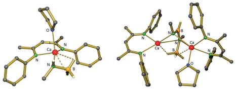
Fig. 5 Crystal structure of compound **11-Me** (I) and its thermal decomposition product **12-Me** (r), displaying the [NMe-BH-NMe-BH<sub>3</sub>]<sup>2-</sup> dianion. <sup>i</sup>Pr groups and most H atoms are omitted for clarity
