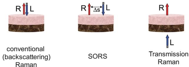
Fig. 1 Schematic diagrams of basic Raman spectroscopy modalities: conventional backscattering Raman, SORS and Raman transmission geometries. Legend: R – Raman light, L – laser beam,  $\Delta s$  – spatial offset.
