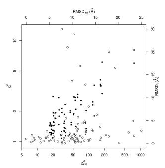
Fig. 2 Benchmark results for SREFLEX<sub>auto</sub> as distribution of  $\chi^2$  and RMSD values. For each case in the benchmark set, a point is drawn using the initial value as abscissa and final value as ordinate, for RMSD (black dots) and  $\chi^2$  (empty circles). The axes corresponding to  $\chi^2$  values are in logarithmic scale.
