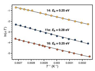
Fig. 6 Comparison of activation energies for non-porous polymers 11a (blue) and 14 (yellow), and porous polymer 16 (red).
