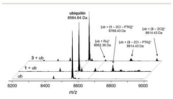
Fig. 5 Deconvoluted nESI-Q-TOF mass spectra of ubiquitin (8564.64 Da) and after incubation with  $\bf 1$  or  $\bf 3$  for  $\bf 48$  h. The mixture was incubated at a  $\bf 2:1$  metal-to-protein ratio in water.
