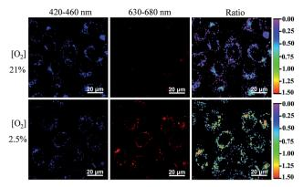
Fig. 3 Confocal luminescence imaging and ratiometric luminescence imaging ( $\lambda_{ex}$  = 405 nm) of HepG2 cells incubated with the FP-Pdots (10  $\mu g$  mL<sup>-1</sup>) at 21% or 2.5% O<sub>2</sub> concentrations. In luminescence imaging, the emission channels at wavelengths of 420-460 nm and 630-680 nm were collected. In ratiometric imaging, the ratio of emission intensity at 630-680 nm to that at 420-460 nm was chosen as the detected signal.
