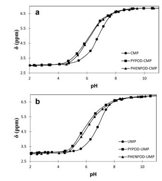
Fig. 4 Plot of <sup>31</sup>P NMR  $\delta$  (ppm) vs. pH for free mononucleotides ( $\bullet$ ) CMP (a) and UMP (b) and for the complexes formed with PYPOD ( ) and PHENPOD (▲).
