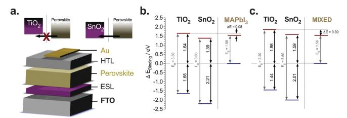
Fig. 1 Energy level diagrams and electron injection characteristics of  $SnO_2$  and  $TiO_2$ -based planar PSCs. (a) Schematic conduction band diagram of the perovskite films and the electron selective layers,  $TiO_2$  and  $SnO_2$  for (b) MAPbI<sub>3</sub> and (c) (FAPbI<sub>3</sub>)<sub>0.85</sub>(MAPbBr<sub>3</sub>)<sub>0.15</sub>, labeled as 'mixed'.
