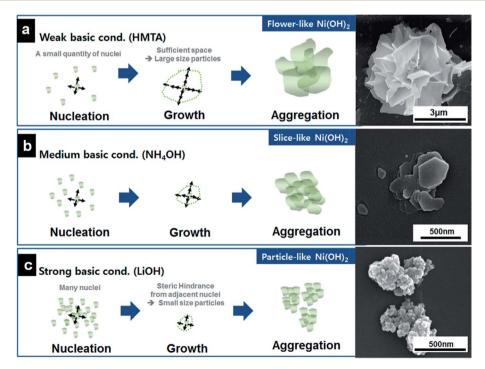
Fig. 22 Schematic diagram showing the formation process of (a) flower-, (b) slice-, and (c) particle-like Ni(OH)<sub>2</sub> under different pH conditions; corresponding SEM Images of as-prepared samples are in the Right Panel. Reproduced with permission from ref. 244. Copyright 2013 American Chemical Society
