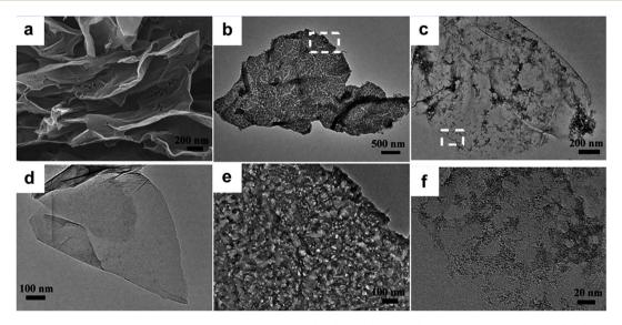
Fig. 15 (a) SEM images of rGO electrode materials. TEM image of rGO (b), rGO-PANi (c and d) and rGO-RuO<sub>2</sub> (e-f). Reproduced with permission from ref. 174. Copyright 2011 The Royal Society of Chemistry.
