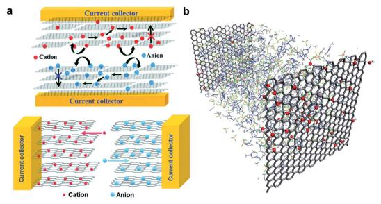
Fig. 12 (a) Conventional stacked geometry used for carbon based electrode material (top) and in-plane supercapacitor configuration made of graphene electrodes (bottom). The schematic depicts the mechanisms of increase in electrolyte percolation for higher performance. (b) Representation of a supercapacitor model consisting of GO electrodes (10% oxidation) with pure EMI+BF4-. Reproduced with permission from ref. 130 and 133. Copyright: 2011 and 2014 American Chemical Society.
