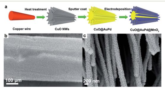
Fig. 8 (a) Schematic illustration of the fabrication process of CuO@AuPd@MnO<sub>2</sub> NWs. (b) SEM image shows that the copper wire is completely covered by CuO NWs. (c) SEM image of MnO2 that was uniformly electrodeposited onto NWs. Reproduced with permission from ref. 83. Copyright 2014 WILEY-VCH Verlag GmbH & Co. KGaA, Weinheim.
