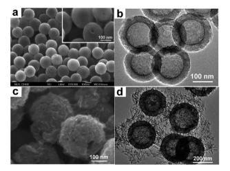
Fig. 5 (a) FESEM and (b) TEM images of HCS-PANI. (c) FESEM and (d) TEM images of GHCS-MnO<sub>2</sub>. Reproduced with permission from ref. 37 and 38. Copyright: 2010 American Chemical Society and 2012 The Royal Society of Chemistry.
