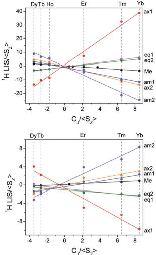
Fig. 6 Reilley plots (Method A) for the proton shifts of LnDTMA in  $D_2O$  at 298 K without added fluoride (top) and for the fluoride-bound species (bottom).
