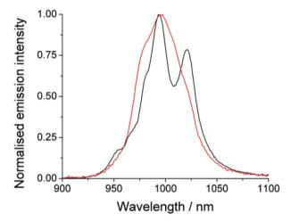
Fig. 1 Change in form of emission spectra with fluoride. Top: EuDTMA in  $D_2O$  (black) and with excess sodium fluoride (red),  $\lambda_{ex}$  = 394 nm, exit slit = 1 nm; inset shows the change in structure of the  $\Delta J$  = 1 band measured with 0.2 nm exit slit. Bottom: YbDTMA in D2O (black) and with added fluoride (red),  $\lambda_{ex}$  = 265 nm, exit slit = 5 nm.
