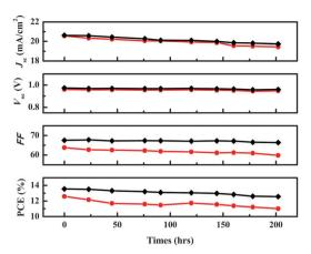
Fig. 4 Time-course changes in the performance parameters of the solar cells with **DPEDOT-B[BMPDP]<sub>2</sub>** (●) and **spiro-OMeTAD** (♦) as the HTMs under inert conditions at room temperature.
