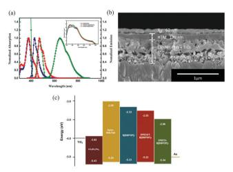
Fig. 2 (a) Absorption and emission spectra of the HTMs in chlorobenzene. Inset: UV-vis absorption spectra of the HTMs coated on mp-TiO<sub>2</sub>/MAPbl<sub>3</sub> films. (b) Cross-sectional field-emission scanning electron microscopy (FE-SEM) image of mp-TiO<sub>2</sub>/MAPbl<sub>3</sub>/HTM/Au. (c) Energy level diagram of each component.
