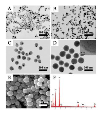
Fig. 1 TEM images of (A) OA-modified Fe<sub>3</sub>O<sub>4</sub> NPs, (B) CTAB-stabilized  $Fe_3O_4$  NPs, (C) eccentric  $Fe_3O_4$ @PAA core-shell NPs, and (D) Fe<sub>3</sub>O<sub>4</sub>@PAA/AuNCs/ZIF-8 core-shell NPs; (E) SEM image of Fe<sub>3</sub>O<sub>4</sub>@PAA/AuNCs/ZIF-8 core-shell NPs; (F) energy dispersive X-ray spectrum of Fe<sub>3</sub>O<sub>4</sub>@PAA/AuNCs/ZIF-8 NPs. Inset in (D) shows the HR-TEM image of part of a single Fe<sub>3</sub>O<sub>4</sub>@PAA/AuNC/ZIF-8 NP.
