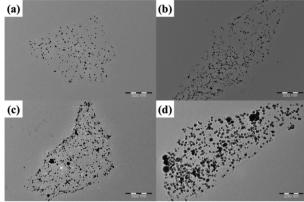
Fig. 5 (a-d) TEM images of RGO/AgNP suspension with different AgNP encapsulations by adjusting the mass ratio of AgNO<sub>3</sub> to GO of about 6:1, 8:1, 10:1, and 12:1, respectively.
