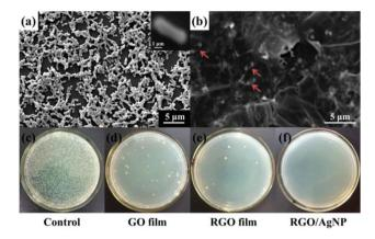
Fig. 8 Antibacterial property of RGO/AgNP hybrid film: (a, b) SEM images of (a) clean silicon wafer (a typical *E. coli* bacterium is shown in the inset) and (b) RGO/AgNP hybrid film on the surface of silicon wafer after the adhesion experiments. (c–f) Photographs of (c) clean silicon wafer, (d) GO film, (e) RGO film, and (f) RGO/AgNP hybrid film after the viability experiments. White areas correspond to bacterial colonies grown during incubation.
