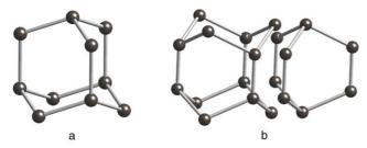
Fig. 1 Basic units (tiles) for (a) diamond and (b) lonsdaleite.
