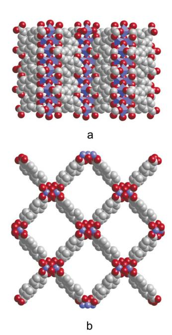
Fig. 4 (a) Impenetrable walls of MOF-69, [100] direction, (b) open channels of MOF-69, [001] direction.
