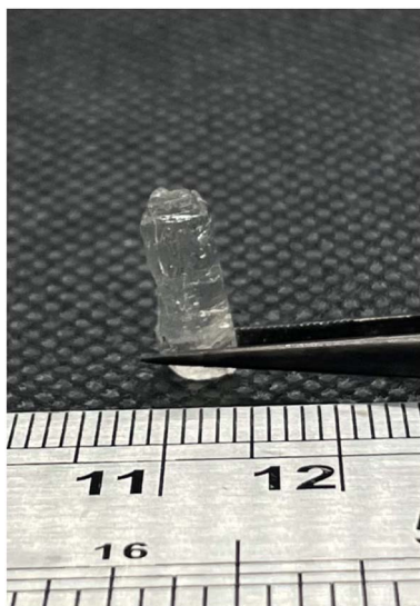
Fig. 7 PG4–Norb (1 : 1) in a larger scaffold produced via photo-polymerization.
