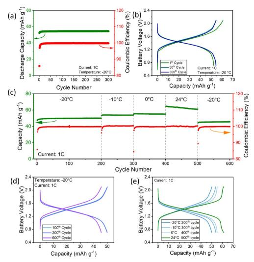
Fig. 7 Long-term cycling results of PNTCDI $\|$ PTMA-co-GMA full cells. (a) Discharge capacity of the cell cycled at -20 °C and 1C (110 mAh g $^{-1}$ ) for 300 cycles. (b) GCD curves of the cell cycled at -20 °C and 1C. (c) The discharge capacity of the cell cycled at different temperatures and 1C current. The GCD curves are also shown in (d) - all taken at -20 °C but different cycle numbers; (e) the last cycle of the GCD curves taken at different temperatures from -20 °C to 24 °C.
