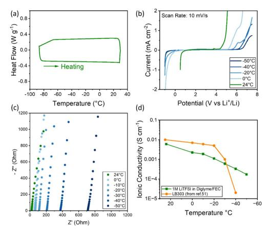
Fig. 1 (a) DSC thermogram of the low-temperature electrolyte (LTE) from -85 °C to room temperature at a scan rate of 10 °C min<sup>-1</sup>. (b) Linear sweep voltammetry of the LTE in a symmetric lithium cell at varying temperatures at a scan rate of 10 mV s<sup>-1</sup>. (c) Nyquist EIS plot of the LTE at different temperatures. (d) Ionic conductivity of the LTE at different temperatures; the ionic conductivity of LB303 (ref. 55) is shown for comparison.
