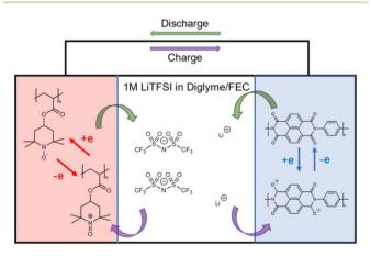
Dual-ion working mechanism
