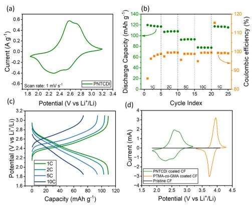
Fig. 2 Electrochemical characteristics of PNTCDI-coated CF in a half cell (vs. lithium foil) at room temperature (24 °C). (a) CV at 1 mV s<sup>-1</sup>. (b) Discharge capacity at varying C-rates. (c) GCD curves at different C-rates. (d) CV curves of PNTCDI, PTMA-co-GMA, and neat CF shown together. The electrolyte was 1 M LiTFSI in diglyme/FEC (9:1, w:w). All cells had an active material loading of >1 mg cm<sup>-2</sup>.
