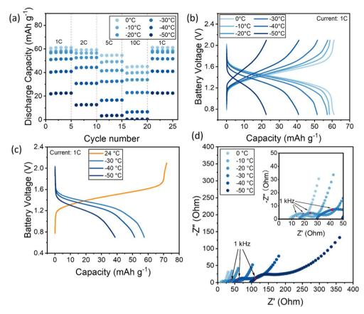
Fig. 6 PNTCDI||PTMA-co-GMA full cell characteristics at low temperatures from -50 °C to 0 °C (a) discharge capacity at current from 1C (110 mA  $g^{-1}$ ) to 10C (1100 mA  $g^{-1}$ ). (b) GCD profiles of the cell at 1C. (c) GCD curves for the cell battery charged at room temperature, kept at 2.1 V while cooling down, and then discharged at various low temperatures. (d) EIS Nyquist plot of the full cell at different temperatures.
