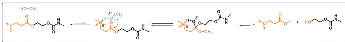
Scheme 1 Proposed mechanism of the transesterification reaction taking place with the BAE-containing compound in the presence of methanol.
