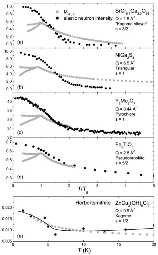
Fig. 4 Neutron scattering intensity (black circles)<sup>36,47,104–106</sup> and magnetic susceptibility (grey circles)<sup>36,45,47,74,104</sup> for various GF compounds as a function of temperature.
