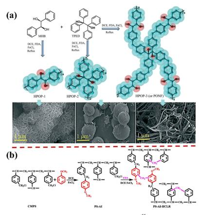
Fig. 10 (a) Schematic of MHB- and TPED-based HCPs and different surface morphology.<sup>66</sup> Copyright 2022, The Royal Society of Chemistry. (b) Synthetic procedure of anisole-modified hyper-cross-linked resins. 71 Copyright 2020, Elsevier.
