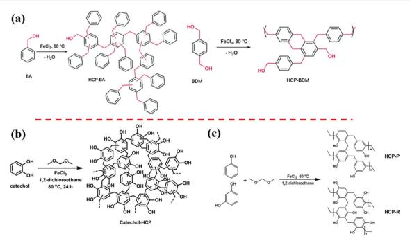
Fig. 8 (a) Synthesis of HCP-BA and HCP-BDM based on a Friedel-Crafts alkylation reaction catalyzed self-condensation.<sup>130</sup> Copyright 2013, The Royal Society of Chemistry. (b) The scheme of catechol-based HCP.<sup>53</sup> Copyright 2020, Springer. (c) Fabrication of hypercrosslinked hydroxyl-rich polymer (HCP-P and HCP-R).<sup>56</sup> Copyright 2020, Elsevier.
