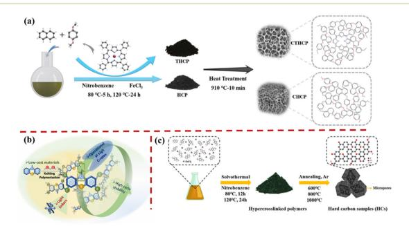
**Fig. 14** (a) Synthesis of hyper-crosslinked polymer-based hard carbon samples. <sup>146</sup> Copyright 2024, Elsevier. (b) Hypercrosslinked phenothiazine polymer as an organic cathode for lithium batteries. <sup>147</sup> Copyright 2024, American Chemical Society. (c) Synthesis of hard carbon anodes for potassium-ion batteries. <sup>119</sup> Copyright 2022, American Chemical Society.
