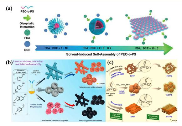
Fig. 11 (a) Solvent-induced self-assembly strategy to produce PEO-b-PS-based porous polymers. 134 Copyright 2019, Wiley-VCH. (b) Synthesis processes of hierarchical nanoporous polymers via the Friedel-Crafts reaction polycondensation. 135 Copyright 2019, American Chemical Society. (c) Synthesis of SCTPS through a Scholl reaction using chloroform at 60 °C for 24 h. 47 Copyright 2022, American Chemical Society.
