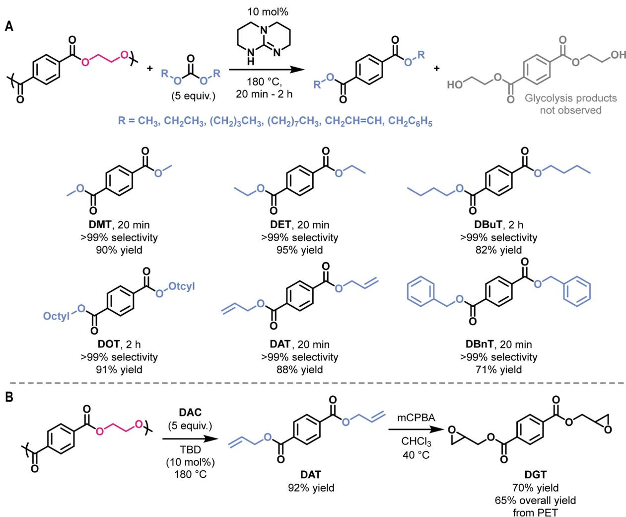
**Fig. 4** (A) High value terephthalate products accessible *via* CID. Reaction conversions and isolated yields are shown below each synthesized compound. (B) Synthesis of diglycidyl terephthalate (**DGT**) in two steps starting from PET egg carton waste.
