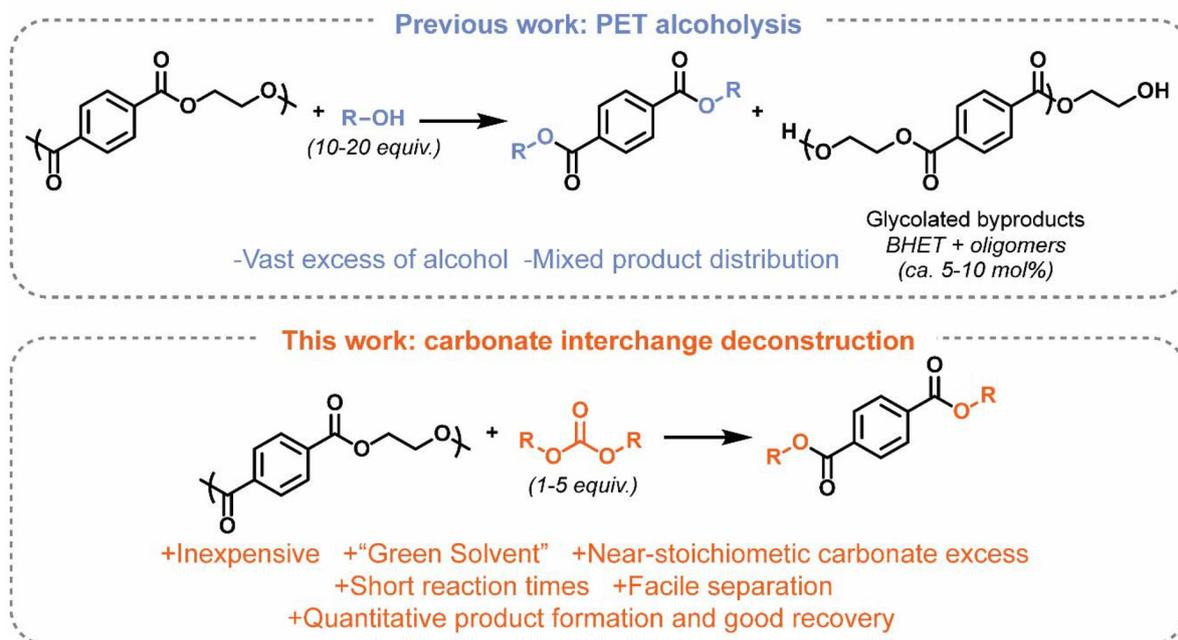
**Fig. 1** (Top) PET deconstruction *via* alcoholysis currently requires vast excesses of alcohol and produces glycolated byproducts. (Bottom) The use of carbonates in place of alcohols for PET deconstruction significantly reduces solvent excess, affording high isolated yields of valuable terephthalate products.
