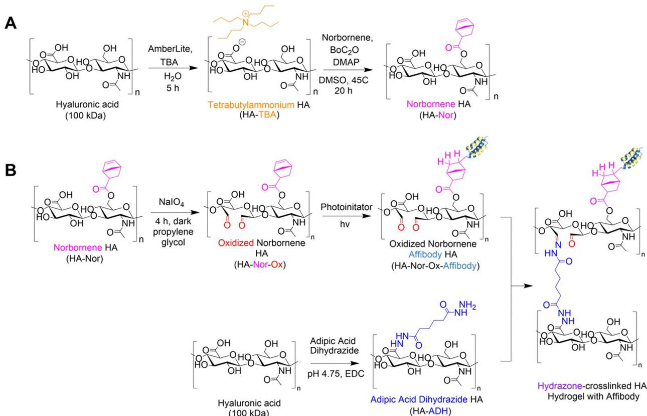
Fig. 5 Synthesis of HA-Nor, HA-Nor-Ox, and HA-Nor-Ox-Affibody. (A) HA was functionalized with a norbornene group through BoC<sub>2</sub>O activated coupling prior to oxidation resulting in HA-Nor-Ox. (B) HA-Nor-Ox was then used to bioconjugate our BMP-2 affibody to the norbornene group through a photoinitiated reaction and thiol-ene click chemistry. The product was then crosslinked with HA-ADH to form a hydrzone-crosslinked hydrogel containing affibodies.
