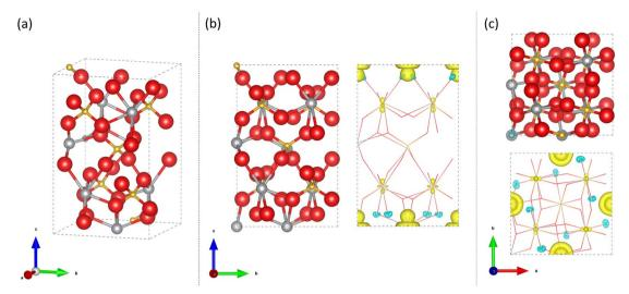
Fig. 10 Calculated structure for 12.5 at% Mo doping of a V site in tetragonal scheelite BiVO₄ for a single unit cell showing atomic positions and spin density [Bi = silver, V = gold, O = red, Mo = light blue; ionic radii proportions scaled down for visibility]. (a) Angled view, (b) a-axis view and (c) c-axis view
