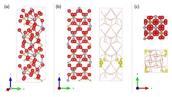
Fig. 9 Calculated structure for 6.25 at% Mo doping of a V site in t-BiVO<sub>4</sub> for a  $2 \times 1 \times 1$  supercell showing atomic positions and spin density [Bi = silver, V = gold, O = red, MO = light blue; ionic radii proportions scaled down for visibility]. (a) Angled view, (b) a-axis view and (c) c-axis view.
