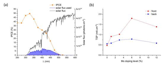
Fig. 8 (a) Calculation of the theoretical solar photocurrent (TSP) for 6% Mo-BiVO<sub>4</sub> under front irradiation at 1.23 V<sub>RHE</sub> and (b) a summary of the TSP photocurrents at 1.23 V<sub>RHE</sub> for front and back irradiation as a function of Mo precursor doping level (%) of BiVO<sub>4</sub> and all Mo-doped BiVO<sub>4</sub> samples.
