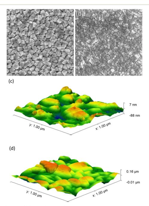
Fig. 4 SEM images of (a) BiVO<sub>4</sub> and (b) 6% Mo-BiVO<sub>4</sub> taken at 50k magnification [the width of each image represents a distance of 3.8  $\mu$ m]. AFM images, of (c) BiVO<sub>4</sub> and (d) 6% Mo-BiVO<sub>4</sub> measured over a 1  $\mu$ m × 1  $\mu$ m square area.
