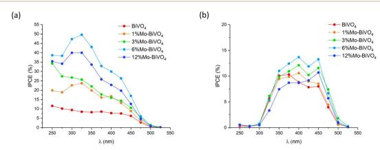
Fig. 7 Incident photon to current efficiency (IPCE) curves for BiVO<sub>4</sub> and all Mo-doped BiVO<sub>4</sub> samples measured with (a) front irradiation and (b) back irradiation. Samples were measured in 0.1 M phosphate buffer (pH = 7) at 1.23  $V_{RHF}$ .
