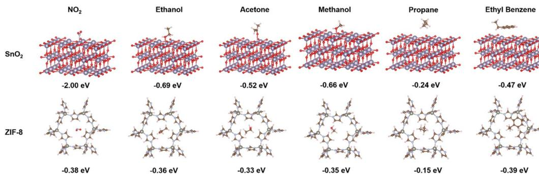
Fig. 4 Density functional theory (DFT) calculations of the adsorption energy of the target gas molecules on SnO<sub>2</sub> and ZIF-8 surface for nitrogen dioxide (NO<sub>2</sub>), ethanol (EtOH), acetone (Ace), methanol (MeOH), propane (Prop) molecules and ethyl benzene (EtBz).
