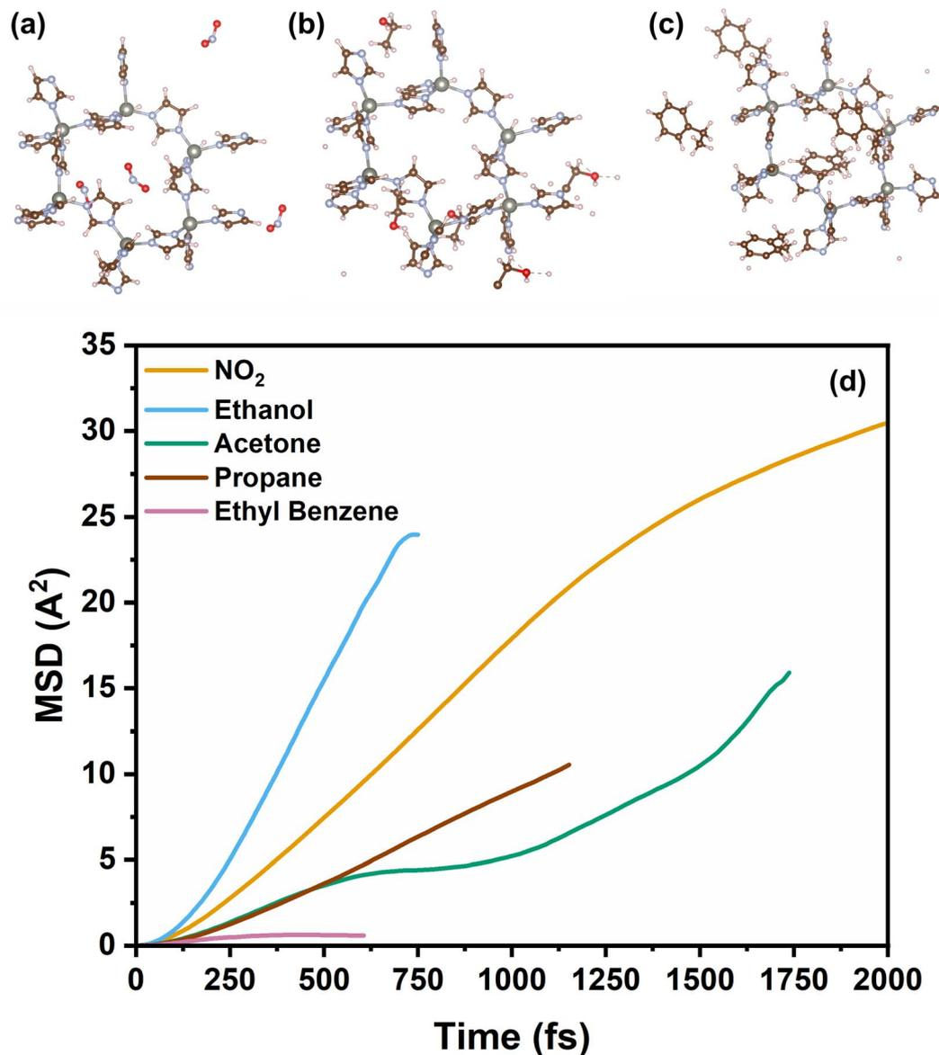
Fig. 7 Molecular dynamic (MD) simulation snapshots of (a) NO<sub>2</sub>, (b) ethanol, (c) ethyl benzene through bulk ZIF-8 membrane before breaking down into smaller molecules. (d) Mean square displacement (MSD) plot of various gases through ZIF-8 membrane.
