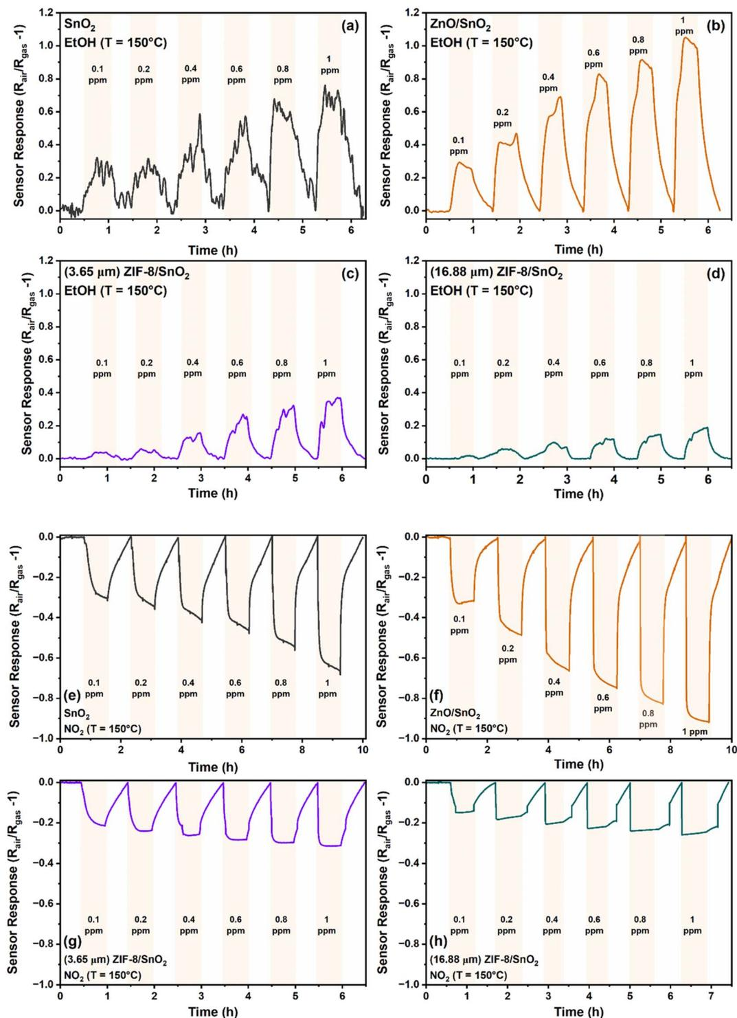
Fig. 3 Dynamic sensing of a pure  $\text{SnO}_2$  layer (black),  $\text{ZnO}/\text{SnO}_2$  dual layer (brown),  $3.65 \mu\text{m}$  ZIF-8/ $\text{SnO}_2$  (purple) and  $16.88 \mu\text{m}$  thick ZIF-8/ $\text{SnO}_2$  (green) dual layer under exposure to increasing concentrations of ethanol, a reducing gas (a–d) and  $\text{NO}_2$ , an oxidizing gas (e–h), from 0.1–1 ppm at an operating temperature of  $150^\circ\text{C}$ .
