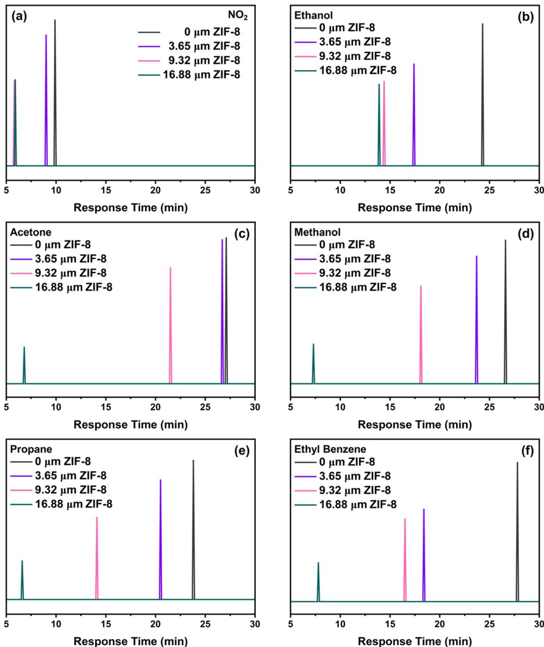
Fig. 6 Response time profiles of the developed sensors with different ZIF-8 thickness: 0  $\mu\text{m}$  (grey), 3.65  $\mu\text{m}$  (purple), 9.32  $\mu\text{m}$  (pink) and 16.88  $\mu\text{m}$  (green) against various target gases (a)  $\text{NO}_2$ , (b) ethanol (c) acetone (d) methanol (e) propane (f) ethyl benzene.
