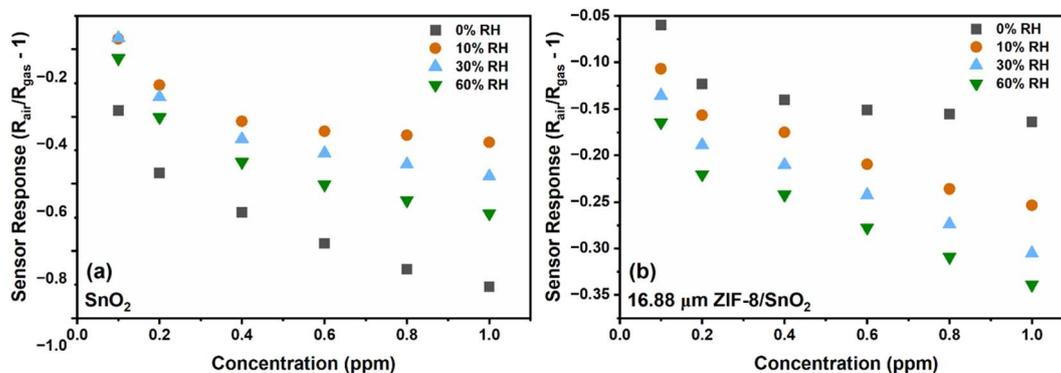
Fig. 9 Effect of different levels of relative humidity (0–60%) on the response of (a) SnO<sub>2</sub> and (b) 16.88  $\mu\text{m}$  ZIF-8/SnO<sub>2</sub> sensors to NO<sub>2</sub> at concentrations ranging between 0.1–1 ppm. All measurements were performed at 150 °C.
