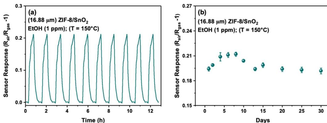
Fig. 8 (a) Reproducibility for 10 cycles (b) long-term stability tests of 16.88  $\mu\text{m}$  ZIF-8/SnO<sub>2</sub> towards 1 ppm EtOH (Ethanol) at 150 °C.
