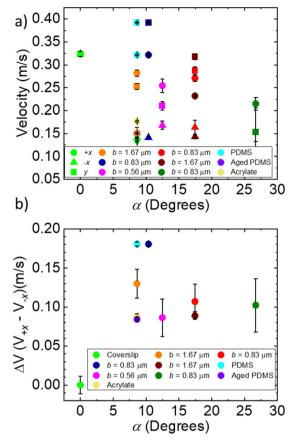
Fig. 4 (a) Droplet velocities vs.  $\alpha$  droplets were blown in the three primary directions +x, -x, y. (b) Difference in velocity between +x and -xdirections
