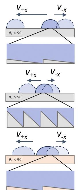
Fig. 6 (top) Low angled surfaces have anisotropic pinning with high velocities in the +x direction and low velocity in the -x direction. (middle) High angled surfaces show strong pinning in both directions with low droplet velocities in the +x and -x directions. (bottom) Hydrophilic surfaces with anisotropic pinning with lower contact angles and velocities.
