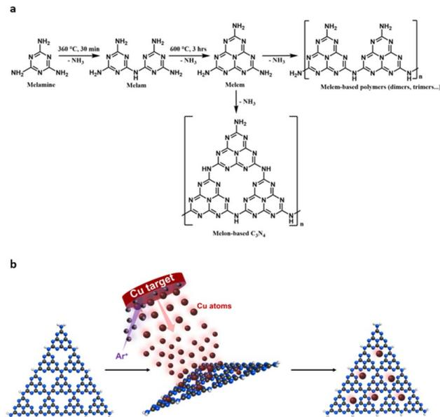
**Fig. 7** (a) Synthesis of b-C<sub>3</sub>N<sub>4</sub> from melamine via a two-step calcination method. Polycondensation under these conditions can yield melam- and/or melon-based polymers. (b) Schematic representation of Cu atoms deposition by sputtering metal atoms from the solid metal target in vacuum directly onto carbon nitride (copper red, carbon grey, nitrogen blue, hydrogen white).
