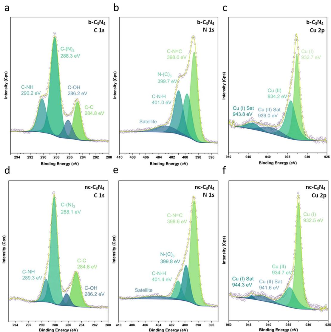
Fig. 2 HR XPS spectra of Cu/b-C<sub>3</sub>N<sub>4</sub> in the C 1s (a), N 1s (b) and Cu p<sup>3/2</sup> (c) regions and Cu/nc-C<sub>3</sub>N<sub>4</sub> in the C 1s (d), N 1s (e), and Cu p<sup>3/2</sup> (f) regions. The raw data (purple circles) is fitted with peaks of oxidation states and satellites in a fitted envelope (yellow).
