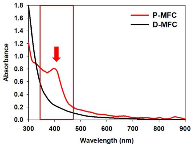
Fig. 2 UV-vis absorption spectra of planktonic and electrode-attached cells on day 9 of the enrichment phase. The red arrow and box indicate that a 400 nm peak only appeared in P-MFC.
