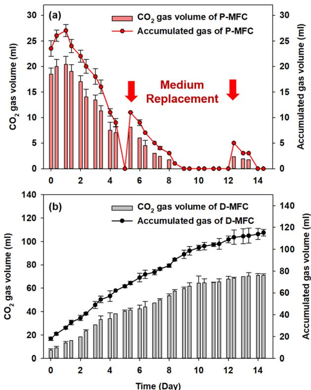
Fig. 5 (a) Accumulated biogas and CO<sub>2</sub> gas volume in the anode chamber after the enrichment phase of P-MFC, and (b) of D-MFC from the second batch cycle with the starting time set to day 0. The red arrows indicate the medium replacement of the P-MFC.
