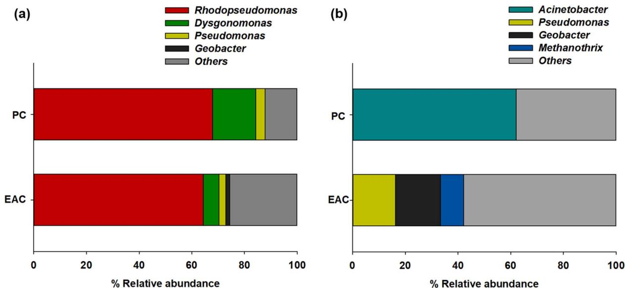
Fig. 3 Relative abundance of major taxonomic groups of (a) P-MFC and (b) D-MFC on day 9 of the enrichment phase. Abbreviations: EAC (electrode attached cells), PC (planktonic cells).
