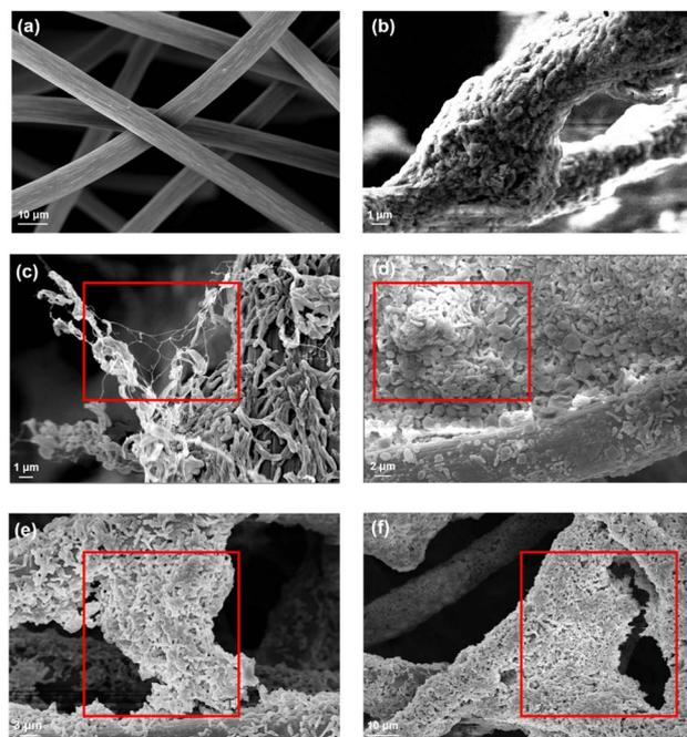
Fig. 6 FE-SEM images of (a) bare graphite felt fiber, and (b) anode-attached cell of D-MFC, and (c–f) P-MFC after the enrichment phase (on day 14). The red box indicates a more aggregated form between cell-to-cell rather than cell-to-anode in the P-MFC.
