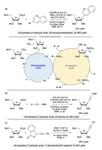
Scheme 16 Photocatalytic, decarboxylative couplings of glycosyl-1carboxylates with (a) bromoarenes;51 (b) alkynes;53 and (c) alkynyliodine(III) reagents.54 bpy denotes 2,2'-bipyridine; Ir-1 denotes [Ir(dF(CF<sub>3</sub>) ppy)<sub>2</sub>(dtbbpy)]PF<sub>6</sub>; chxn denotes trans-1,2-diaminocyclohexane; Ir-2 denotes [Ir(dF(CF<sub>3</sub>)ppy)<sub>2</sub>(d(CF<sub>3</sub>)bpy)]PF<sub>6</sub>.
