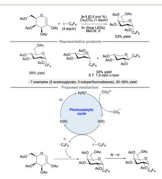
Scheme 49 Synthesis of perfluorinated C-glycosides by photocatalytic radical addition to 2-acetoxyglycals. Ir-1 denotes [Ir(dF(CF<sub>3</sub>) ppy)<sub>2</sub>(dtbbpy)]PF<sub>6</sub>.
