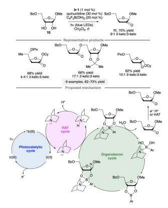
Scheme 55 Redox isomerizations of furanosides to 3-deoxy-2ketosugars. Ir-1 denotes [Ir(dF(CF<sub>3</sub>)ppy)<sub>2</sub>(dtbbpy)]PF<sub>6</sub>; Cy denotes cyclohexyl; Ar denotes pentafluorophenyl.
