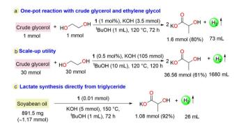
Scheme 2 Practical applicability: (a) conversion of crude glycerol and ethylene glycol to lactate catalyzed by 1; (b) scale-up reaction with crude glycerol and ethylene glycol; (c) one-pot lactate synthesis from triglyceride.
