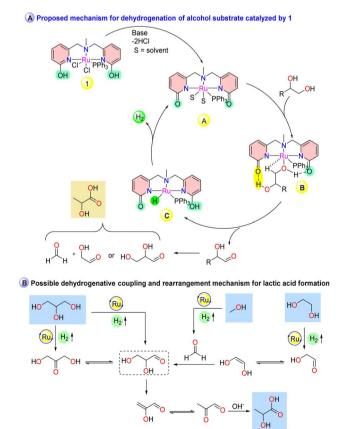
Fig. 1 Proposed mechanism for the dehydrogenation of the alcohol substrate for the synthesis of lactate catalyzed by 1.
