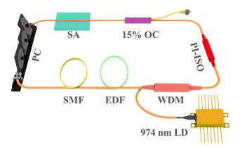
Fig. 5 Schematic diagram of the mode-looked erbium-doped fiber laser.
