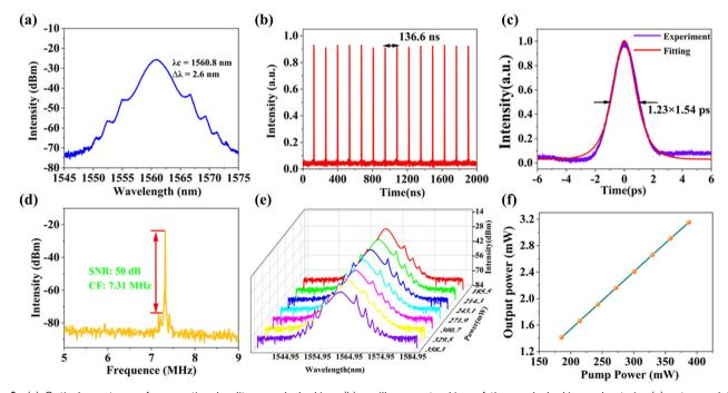
Fig. 6 (a) Optical spectrum of conventional soliton mode-locking; (b) oscilloscope tracking of the mode-locking pulse train; (c) autocorrelation trace with a sech<sup>2</sup> fitting; (d) the RF spectrum of mode-locking pulses; (e) spectral evolution at different pump powers; (f) output power at different pump power.
