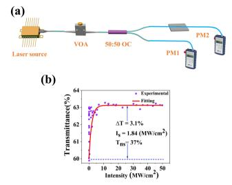
Fig. 4 (a) Installation diagram of Fe-ZIF-67 saturation absorption curve measurement system; (b) the nonlinear transmittance curve.
