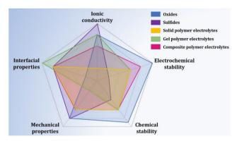
Fig. 12 Comparison of the performance of SSEs with oxide, sulfide, and polymer systems. Reprinted with permission from ref. 153. Copyright 2020 American Chemical Society
