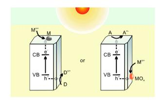
Fig. 1 Schematic diagram of reductive or oxidative photodeposition. VB: valence band, CB: conduction band, M: metal, D: electron donor, A: electron acceptor, and n: number of electrons (or holes) involved.
