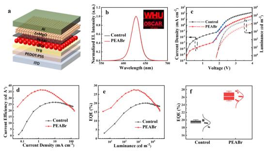
Fig. 2 (a) Schematic diagram of the PEABr-based device structure. (b) Normalized EL spectra. Inset: Photo of two operating PEABr-based QLEDs with different logos. (c) J-V-L, (d) CE, and (e) EQE curves of the device with and without PEABr. (f) Numerical distributions of the EQEs measured from 10 devices, respectively
