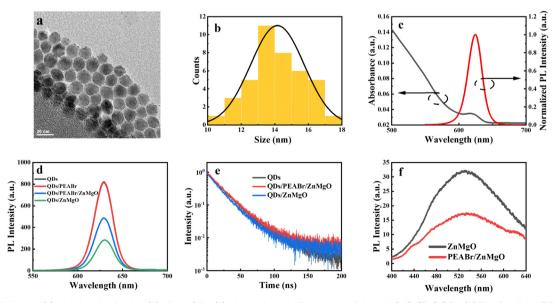
Fig. 1 The TEM image (a) and size distribution (b) of the QDs. (c) Absorption and PL spectra of the red CdSe/ZnS QDs. (d) The PL of the QDs, QDs/PEABr, QDs/PEABr/ZnMgO, and QDs/ZnMgO deposited on quartz, respectively. (e) TRPL of the QDs, QDs/PEABr/ZnMgO, and QDs/ZnMgO, respectively. (f) PL spectra of ZnMgO and PEABr/ZnMgO
