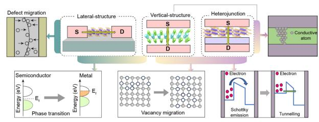
Fig. 3 Schematic depicting common mechanisms of RS. Reproduced with permission from ref. 12. Copyright 2020, John Wiley & Sons, Inc.
