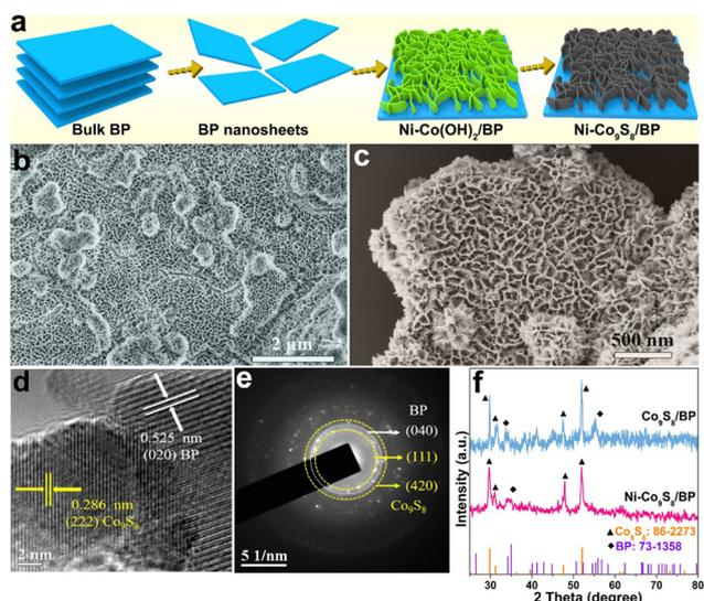
**Fig. 1** (a) Synthesis diagram of the Ni-Co<sub>9</sub>S<sub>8</sub>/BP heterostructure. SEM images of (b) Ni-Co(OH)<sub>2</sub>/BP and (c) Ni-Co<sub>9</sub>S<sub>8</sub>/BP. (d) HRTEM and (e) SAED images of Ni-Co<sub>9</sub>S<sub>8</sub>/BP. (f) XRD patterns of Co<sub>9</sub>S<sub>8</sub>/BP and Ni-Co<sub>9</sub>S<sub>8</sub>/BP, respectively.
