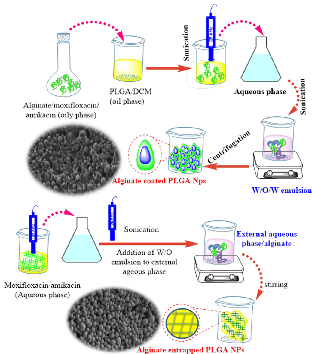
Fig. 4 Schematic presentation of alginate entrapped PLGA nanoparticles and alginate-coated PLGA NPs along with their respective SEM images. 51
