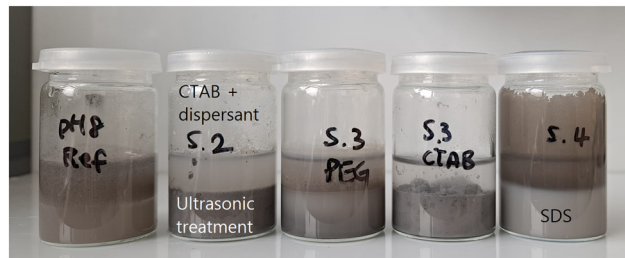
Fig. 6 Five different combinations of surfactants and dispersants in two immiscible liquid systems (top: cyclohexane, bottom: DI water, from left to right: S1–S4) S1: reference mixture at pH 8, S2: CTAB + citric acid and ultrasonic treatment included in the process, S3: PEG and CTAB as a surfactant, S4: SDS as a surfactant.
