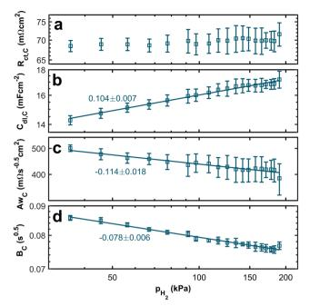
Fig. 7 Double-logarithmic plots of (a) the cathodic charge transfer resistance; (b) the double layer capacitance  $C_{dl,C}$ ; (c) the first Warburg short parameter  $Aw_C$ ; and (d) the second Warburg short parameter  $B_c$
