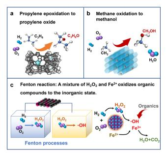
Fig. 12 Schematic diagram of (a) propylene epoxidation to epoxypropane, (c) Fenton reaction, and (b) methane oxidation to methane.
